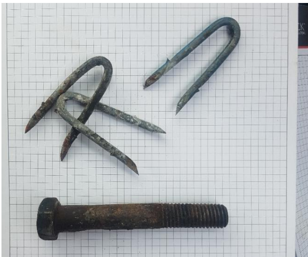
Some of the contaminants collected by the Dimple-Mag™ Extraction System shortly after installation.
